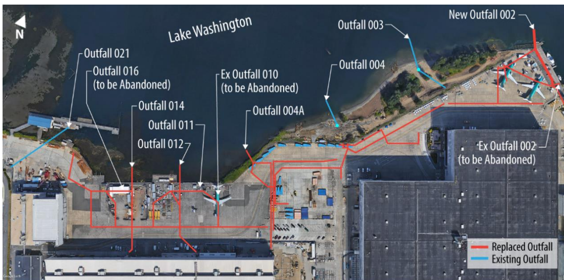
Figure 6. Apron R Stormwater Improvements
