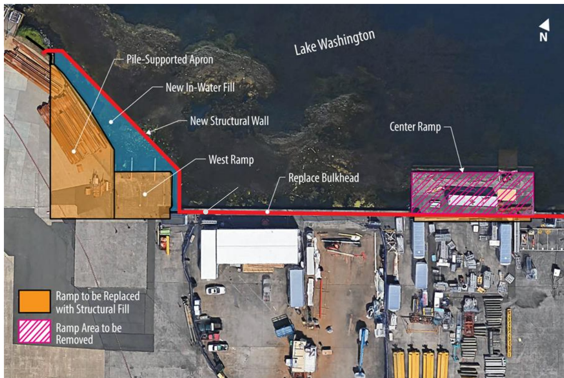
Figure 3. Overwater Structure Removal
